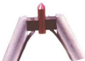
Figure 1.4.1.1: A typical LaB 6 electron source. The LaB 6 is the purple crystal in the centre and is supported under compression with graphite.
