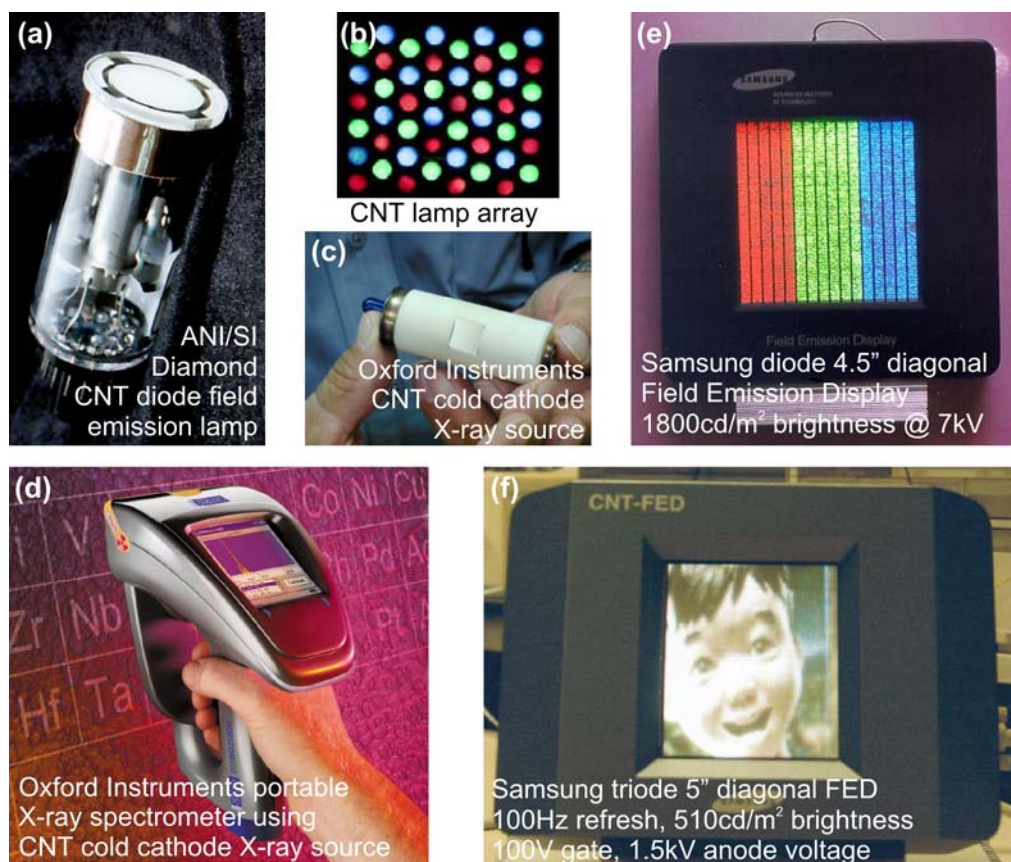
Figure 1.3.2: Applications, such as lamps, X-ray source and field emission displays, using carbon nanotubes (CNT) as the field emission electron source [36].
