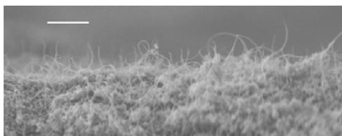
**Figure 6. CNTs Used in Backlight Units (scalebar 1 $\mu$ m)**
