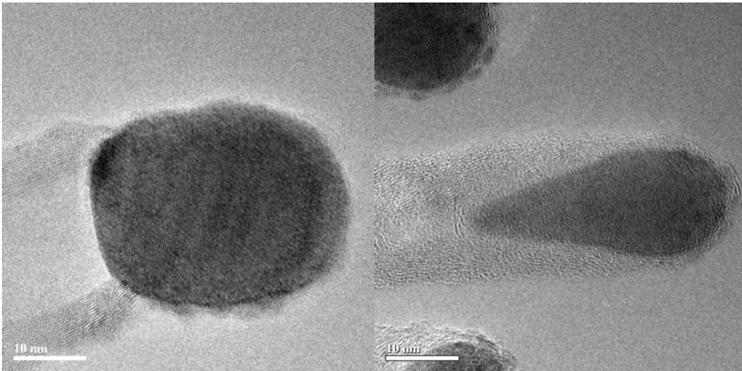
Figure 3: Left, TEM micrograph of the cap of a typical CNT grown from Ni catalyst at 750 °C. Note the disordered and amorphous cap structure without the wall-like graphene structure observed further down. Right, shows a CNT that has been annealed for 6 mins at 1400 K and  $3 \times 10^{-6}$  mBar. Graphene structure is clearly visible all the way around the cap; there is clearly a marked improvement in the CNT as a consequence of the annealing process. Both scale bars are 10 nm.
