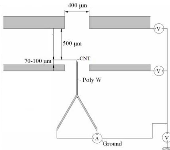
Figure 1: Left, a picture of typical electron suppressor module. Right, a schematic diagram of the set-up used to extract current from the CNT. The piece of metal through which the CNT-W structure protrudes is the suppressor.
