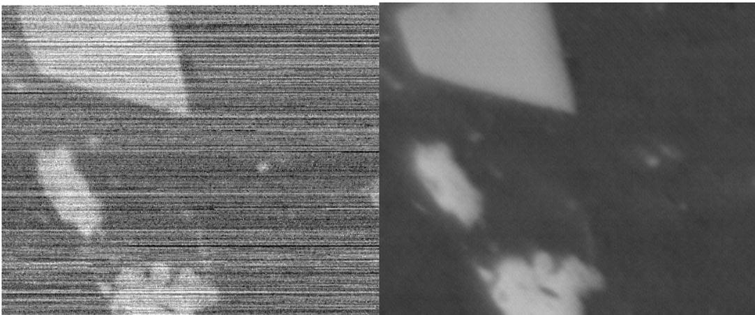
Figure 5: Left, a scanning electron micrograph using a CNT source which can be used to compare the resolution and stability of a typical SFE micrograph shown right. Whilst the CNT image is much noisier, the objects in the image are sharper. Pay particular attention to the improved resolution in the edges of the object with straight sides at the top left of the image. It is otherwise very difficult to see a difference.
