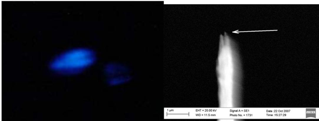
Figure 4: Left, the most stable field emission pattern from the CNT cathode, right, used for microscopy imaging. There appear to be at least five CNTs at the apex. The topmost CNT, indicated by the white arrow, extends significantly higher than the rest. Blurring is due to charging.
