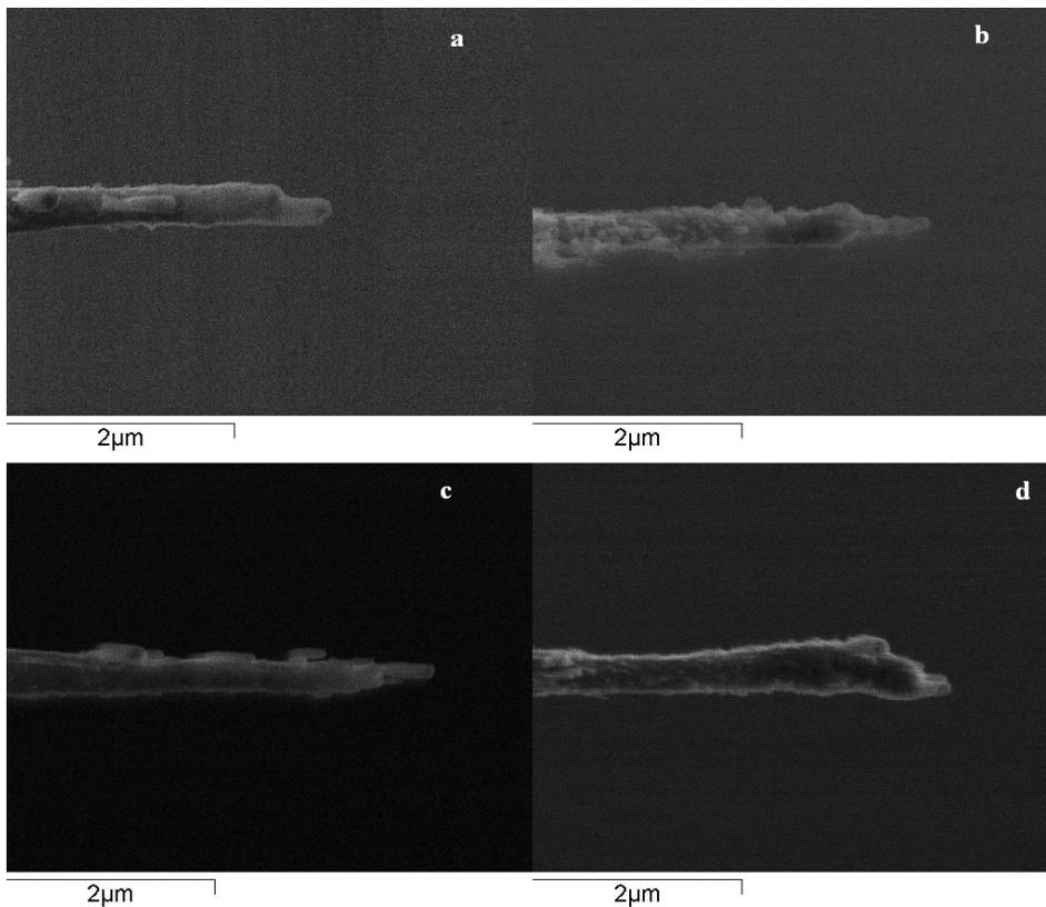
Figure 2: Three single CNTs grown on tungsten tips and a double tip mounted in electron sources. The tips have the following approximate dimensions: (a) length 450 nm, diameter 170 nm (b) length 450 nm, diameter 80 nm (c) length 460 nm, diameter, 80 nm (d) length 240 nm, diameter 70 nm. Note (d) is a double tip with the secondary CNT likely to adversely affect field emission.
