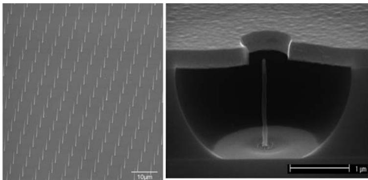
**Figure 3:** (a) Array of MWCNTs of height 5 μm and separation 5 μm [28] (b) Individual MWCNT grown in a micropore etched into SiO<sub>2</sub> using a self alignment method [33].
