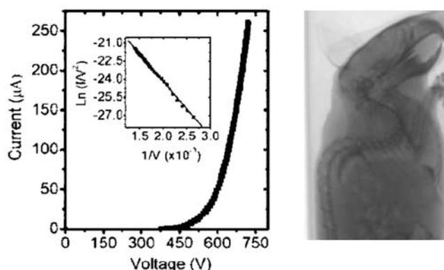
**Figure 9:** Left, the x-ray tube current versus the gate voltage measured with the anode voltage fixed at 40 kV. It follows the classic Fowler–Nordheim relation. The distance between the cathode and the gate is 150  $\mu\text{m}$ . Right, X-ray image of a normal mouse carcass (25 g) obtained using a CNT source-based imaging system [158]. Reprinted with permission from J Zhang, *Rev. Sci. Instrum.* 76, 094301 (2005). Copyright 2005, American Institute of Physics.
