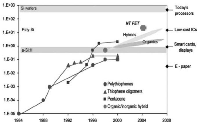
**Figure 12:** The evolution of the mobility of the plastic FET devices over the past decades. The mobility of CNT FETs is indicated by the bold cross towards the top right-hand corner. Some application barriers are also indicated on the right side of the figure [182]. G Gruner. *J. Mater. Chem.*, 2006, 16, 3533 – 3539 – Reproduced by permission of the Royal Society of Chemistry.
