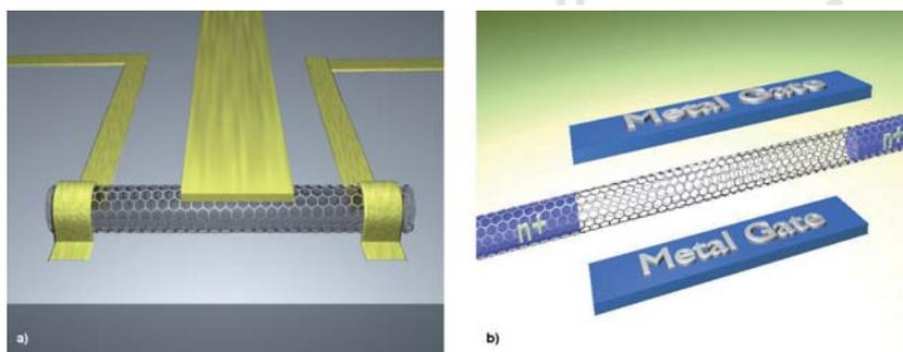
**Figure 1:** Artist's representation of the model for the simulation of a single (a) and a double (b) gate carbon nanotube transistors.
