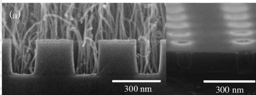
**Figure 11:** Left, CNT vias grown in pores etched into silicon [177], © [2007] IEEE. Reprinted, with permission, from M. Nihei et al., "Electrical Properties of Carbon Nanotube Via Interconnects Fabricated by Novel Damascene Process", Proceedings of IEEE/ IITC 2007. Right, CNTs grown in pores in Silicon.
