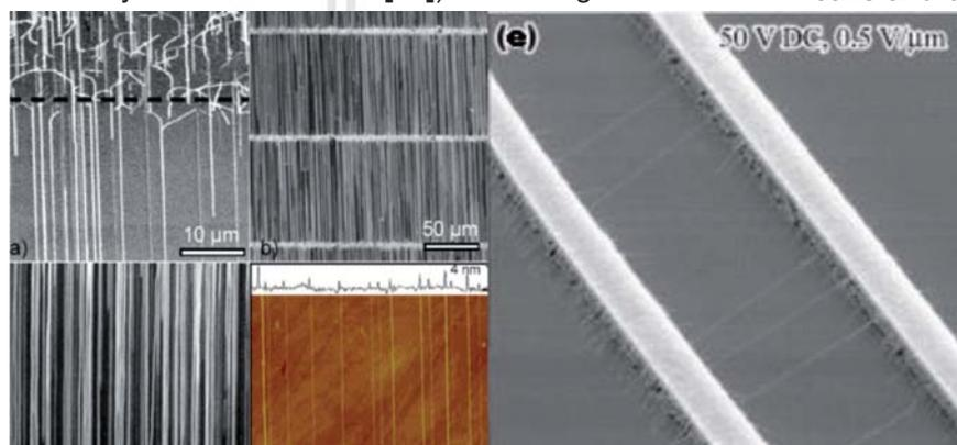
**Figure 4:** (a-d) CNTs grown along quartz crystal planes by the Rogers group [24]. Reprinted with permission from Coskun Kocabas, Moonsub Shim, and John A. Rogers. *J. Am. Chem. Soc.* 2006, 128, 4540-4541. Copyright (2006) American Chemical Society, (e) Horizontally aligned CNTs grown by Dai's group using field to align the CNTs [49]. Reused with permission from Yuegang Zhang, *Applied Physics Letters*, 79, 3155 (2001). Copyright 2001, American Institute of Physics.
