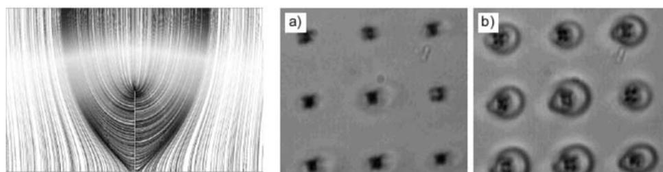
**Figure 16:** Left, Simulated electrical field profile surrounding the single carbon nanotube (10 μm high) with an applied field of 1V m<sup>-1</sup>. Right, Defocus of the nanotube lenslet array at 40x. a) Defocused image of the array at 0 V μm<sup>-1</sup> applied field. b) Array brought into focus with 2.1 V μm<sup>-1</sup> applied field [217].
