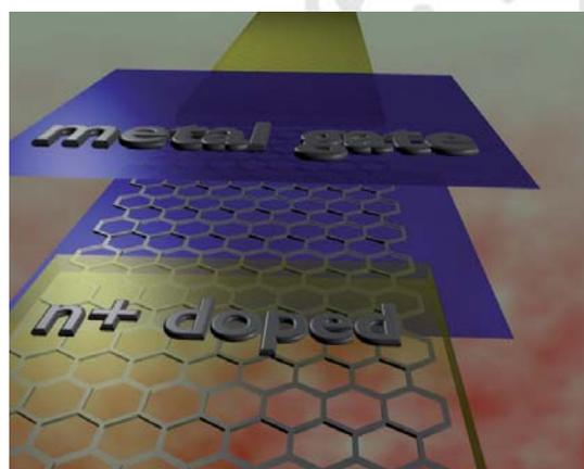
**Figure 2:** Double-gate graphene nanoribbon transistor.
