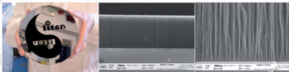
**Figure 5:** Dense forest of Small diameter MWCNT from left to right: a) Patterned layer on a 200mm layer b) 50μm high forest on conductive layer of TiN c) close view of the material with individual CNT making bundles of 60nm of diameter (courtesy of CEA-LITEN).
