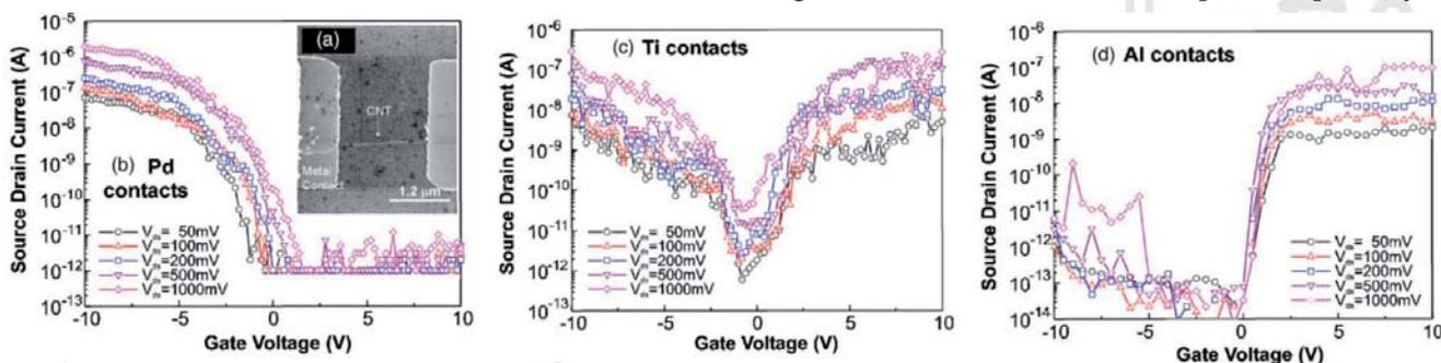
**Figure 13:** SWNT-FET transistor characteristics with different contacts. Left, Pd makes an ohmic contact which results in p-type conduction. Centre, Ti contacts result in strong ambipolar behaviour. Right, Al makes a Schottky contact which results in n-type conduction but with a strong leakage current.
