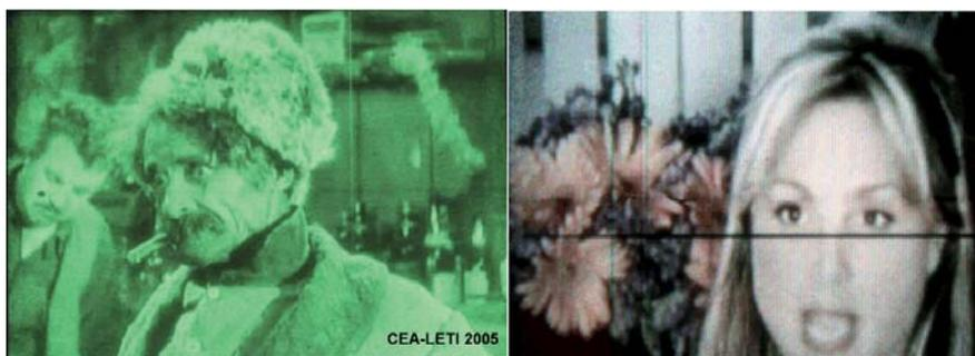
**Figure 7:** Two stages of development of CNT FED at CEA. On the left: monochrome display with  $350\mu\text{m}$  pixels, on the right: color video display with  $600\mu\text{m}$  pixels. On these display the non uniformity from pixel to pixel is 5% while it is 3% with LCD displays and 2% for CRT (courtesy of CEA-LITEN).
