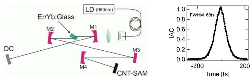
**Figure 15:** Left, Experimental setup of the Er/Yb:glass laser. OC: output coupler; M1-M4: standard Bragg-mirrors; CNT-SAM: Saturable absorber mirror based on carbon nanotubes; LD: pigtailed laser diode for pumping the Er/Yb:glass (QX/Er, Kigre Inc., 4.8 mm path-length). Right, background-free autocorrelation. The solid line is a sech<sup>2</sup> fit with a corresponding FWHM pulse-duration of 68 fs [215].
